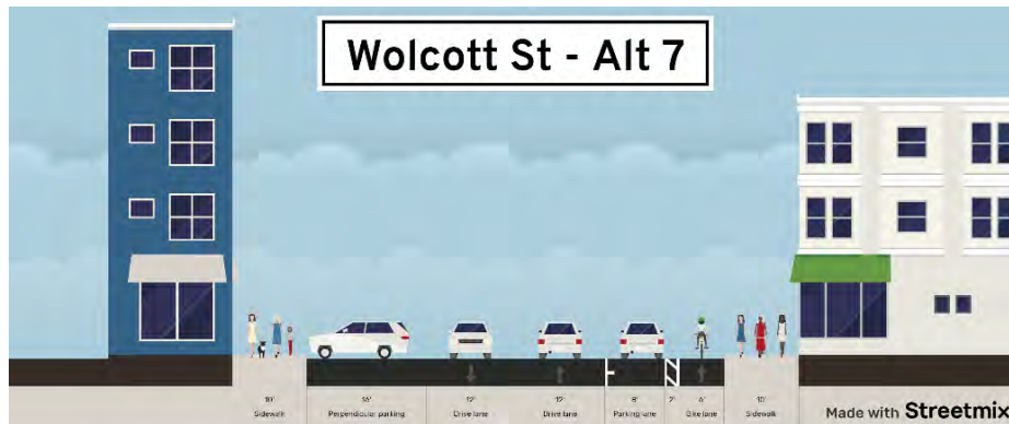
FIGURE 43: WOLCOTT ST ALTERNATIVE 7 PROPOSED CROSS SECTION
