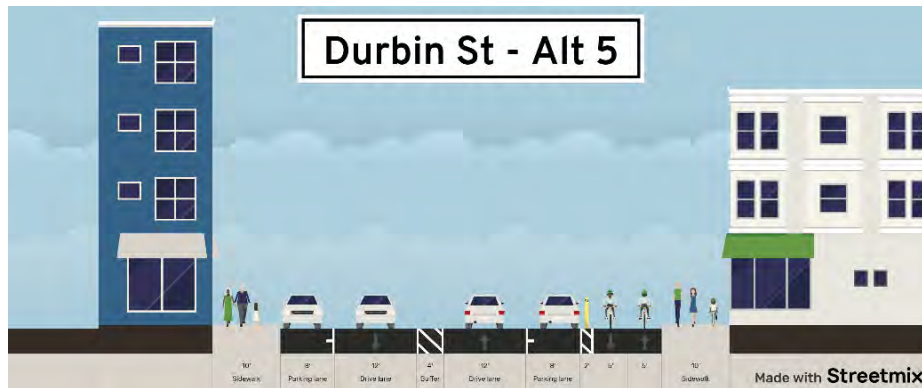
FIGURE 35: DURBIN ST ALTERNATIVE 5 PROPOSED CROSS SECTION
