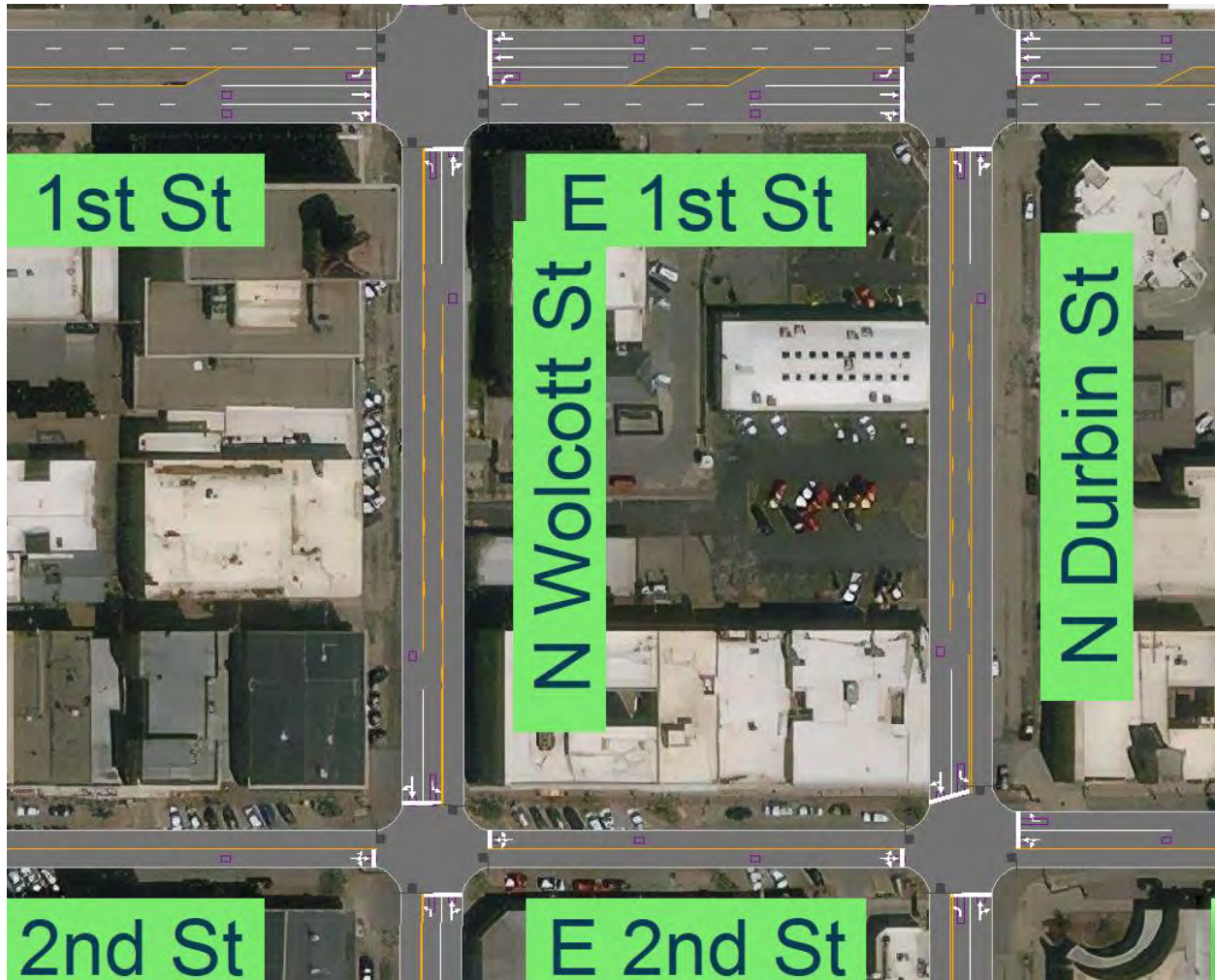
FIGURE 46: CONCEPTUAL TWO-WAY LANE CONFIGURATIONAL AND PAVEMENT MARKING
