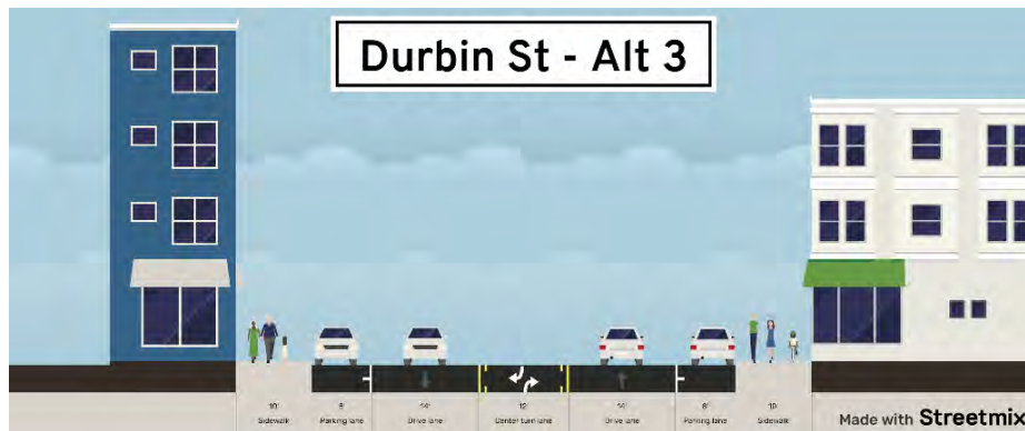
FIGURE 33: DURBIN ST ALTERNATIVE 3 PROPOSED CROSS SECTION
