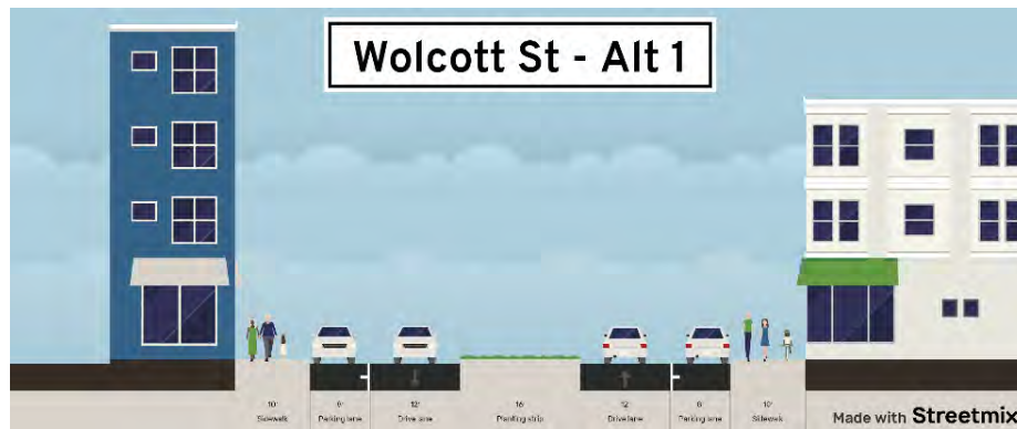
FIGURE 37: WOLCOTT ST ALTERNATIVE 1 PROPOSED CROSS SECTION
