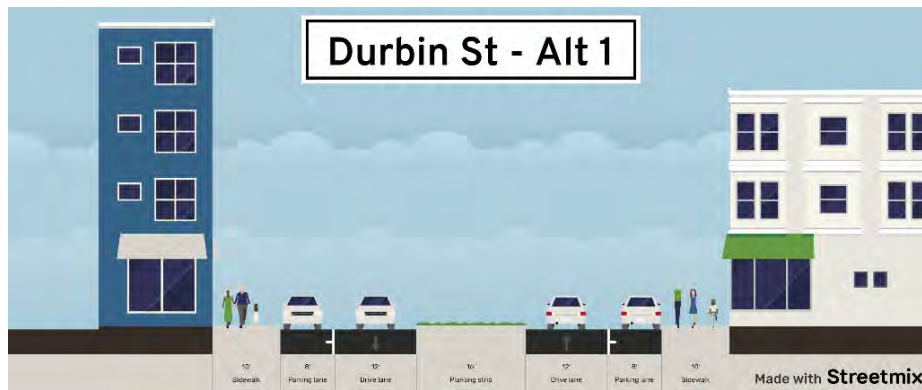
FIGURE 31: DURBIN ST ALTERNATIVE 1 PROPOSED CROSS SECTION
